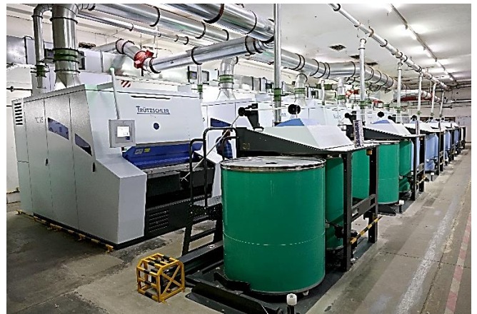
A view of new “Trutzschler – TC 15” Carding Machine installed in our Unit – I at Rajapalayam.
