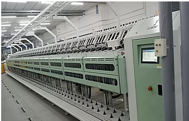
A view of new “LMW-LF 4280A” – Simplex Machine installed in our Unit-II at Subramaniyapuram.
