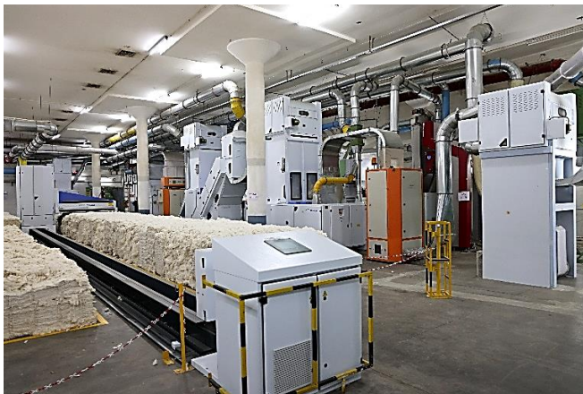
A view of new “Blendomat Trutzschler” Automatic Bale Opener Machine installed in our Unit – I at Rajapalayam.
